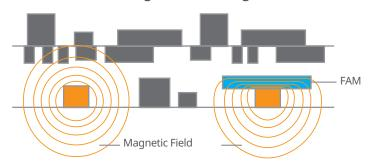
FAM can change the magnetic flux path to avoid the magnetic flux affect others components.
