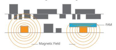
FAM can change the magnetic flux path to avoid the magnetic flux affect others components.
