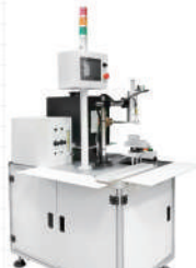
High Frequency Spot Welding Machine
